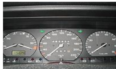
Eddy current speedometers used in automobiles typically have a threshold of about 15 km/h.
